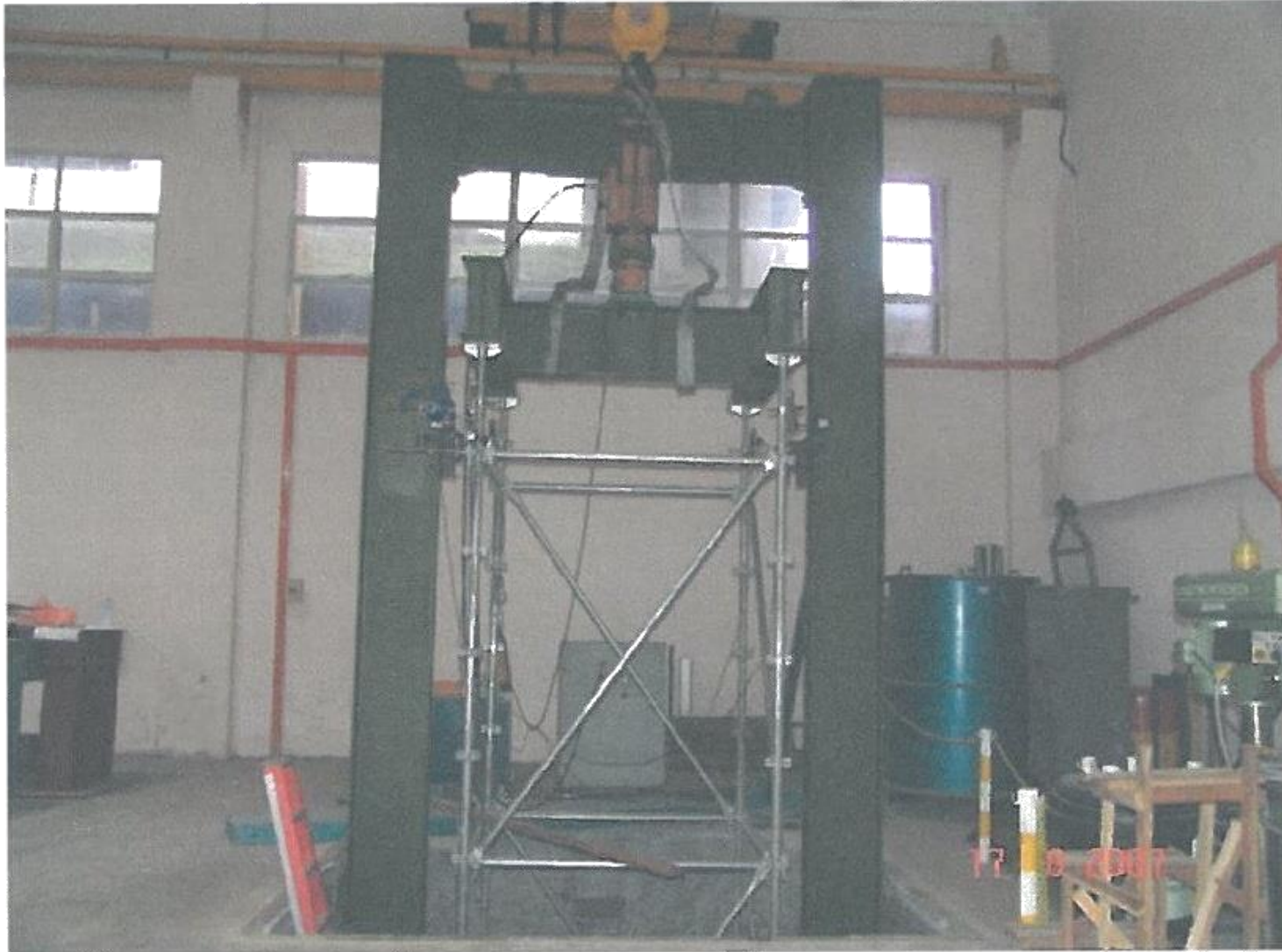
Picture 01: Load test on CRAB 25 modular system scaffold tower (Type 2). 21
