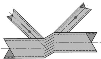
**Mode E: Overall shear failure of the chord**
