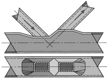
**Mode A: Plastic failure of the chord face**
