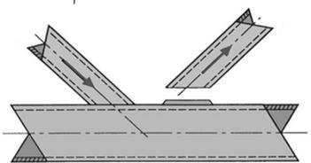
**Mode C: Tension failure of the web member**
