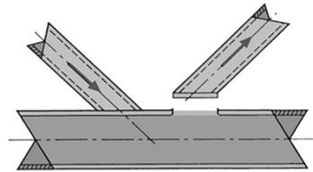
**Mode B: Punching shear failure of the chord face**
